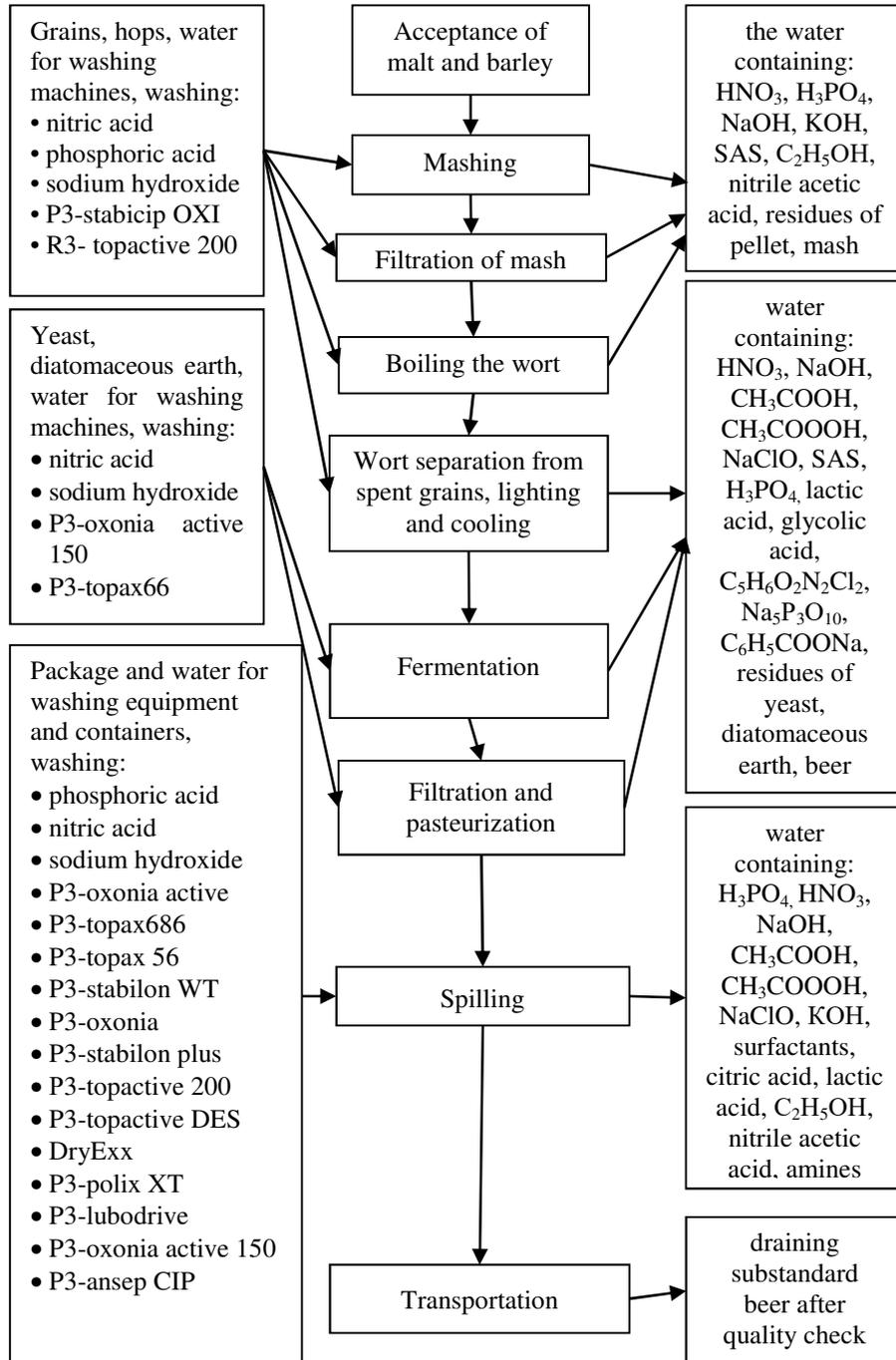
Fig. 2. Scheme of wastewater formation
